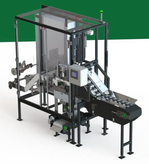
The **AF-40 Potato Wrapper** uses our unique patented belt design to wrap potatoes in aluminum foil at a rate of 40 per minute. This one-of-a-kind machine uses rolls of foil rather than individual sheets. Product is brought in via a servo-operated roller in-feed and dropped softly into catch gates. A photo electric eye triggers the servo-driven plunger to gently drive the product through the pre-cut foil and into the wrapping belts. The wrapped product is deposited onto the discharge conveyor.
